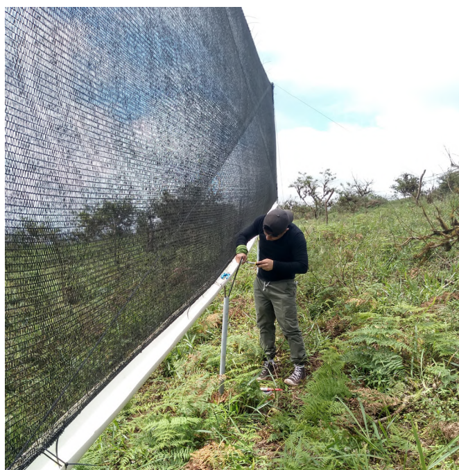
Co-Galápagos interns working to support the largest ever trial of fog-harvesting technology in Galápagos, Credit: Charlie Ferguson
